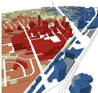
Figure 7. RDI scores connectivity at the parcel level, allowing scores to be related to land use information and other GIS data. In these images, “taller” parcels reflect higher land use density (address points per acre). This image shows Lakewood station area land use density and RDI before improvements. The Sounder station is shown as a green square.
